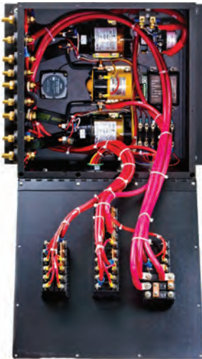
Ignition Protected Main DC power distribution enclosure assembly. Includes: battery switching solenoids, circuit breakers, fuse blocks, relays, external power studs and connectors.
