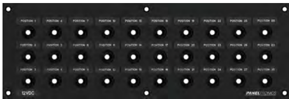
7203 16.50" W x 5.50" H x 2.50" D DC 30 Position Push-to-Reset Circuit Breaker Panel 9997203 Black, 12/24 VDC, Loaded with 30 - 15Amp Push-to-Reset Circuit Breakers
