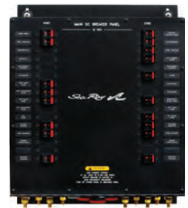
Bulkhead mount Main DC Engine Room Control Panel with enclosure protection. Includes: ignition protected circuit breakers, fire protection control module, external connectors and power studs.
