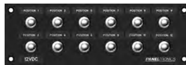
7262 10.50" W x 3.50" H x 2.50" D DC 12 Position Push-to-Reset Circuit Breaker Panel 9997262 Black, 12/24 VDC, Loaded with 12 - 15Amp Push-to-Reset Circuit Breakers
