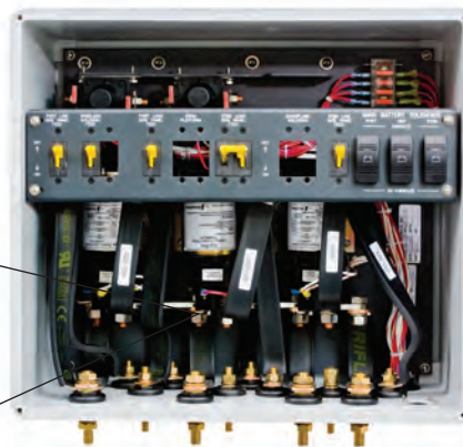
Main DC Power Disconnect and Distribution Enclosure assembly. This assembly is pre-wired with flexible bus bars that permit a higher density in a smaller enclosure. Includes: a NEMA rated fiberglass enclosure, ignition protected circuit breakers, battery switching solenoids, relays, fuse blocks, control modules, and external connectors and power studs.
