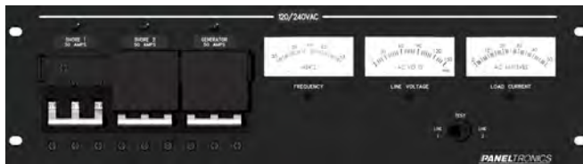
6303 19" W x 5.25" H (3-U) 3 - AC High Amp Mains with Source Selection Sliding Gate Interlock and Meters (available for 120 VAC, 240 VAC - 60 Hz and 220 VAC - 50 Hz)
