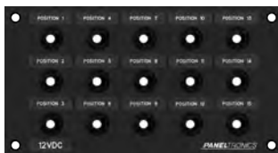
7253 9.00" W x 4.85" H x 2.50" D DC 15 Position Push-to-Reset Circuit Breaker Panel 9997253 Black, 12/24 VDC, Loaded with 15 - 15Amp Push-to-Reset Circuit Breakers
