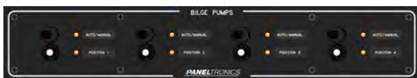
4208 17.75" W x 3.25" H x 3.5" D DC 4 Position Bilge Pump Panel Each Position includes Auto/Manual Switch and Push-to-Reset 15 Amp Circuit Breaker
