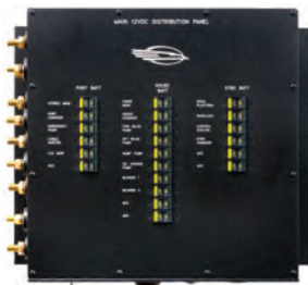
Ignition Protected Main DC power distribution enclosure assembly. Includes: battery switching solenoids, circuit breakers, fuse blocks, relays, external power studs and connectors.
